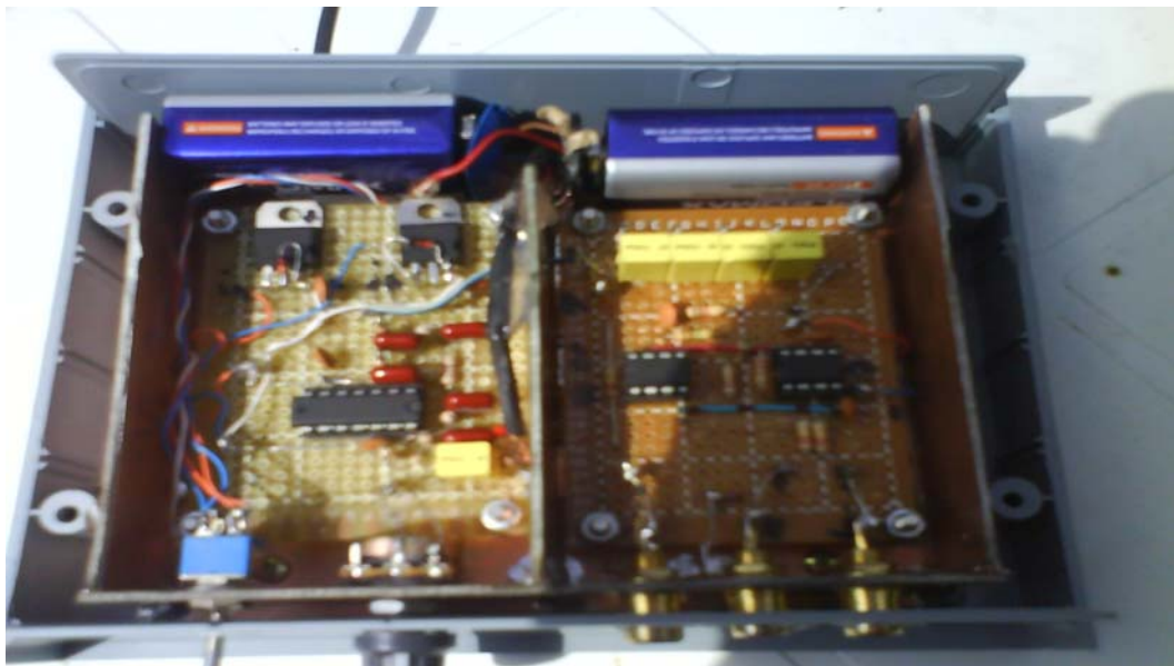
Figure 11. Practical realization of the EKG amplifier
