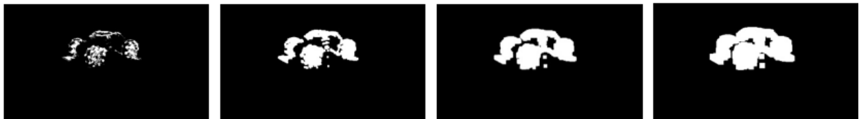
Figure 2. From left to right: the initial mask resulted after the thresholding operation, the mask after the first dilate operation, the mask after the second dilate operation, and the last mask resulted after the third dilate transformation
